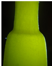
ASTM D638 Type 1 exhibiting improved properties during tensile
